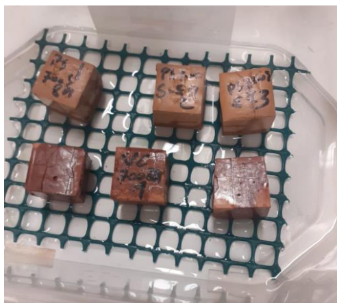
Figure 66- Example of capillary water absorption tests carried out according to UNI EN 10859:2000 on all obtained samples.
