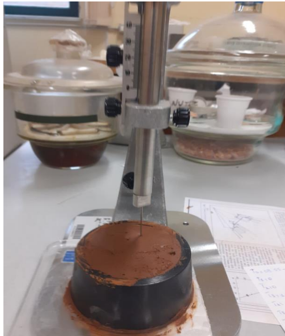
Figure 67 - Vicat Needle test on the samples
