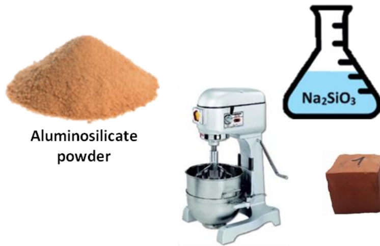
Figure 23- Geopolymer preparation scheme
