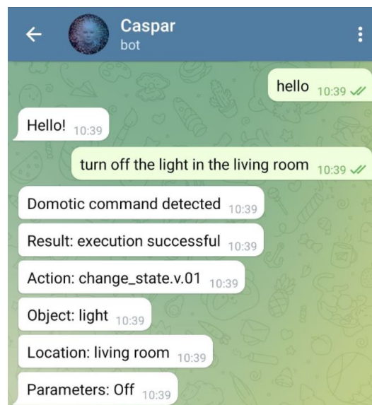
Figure 3.7: AD-CASPAR execution of a Internet of Thing command in a Telegram chat session.
