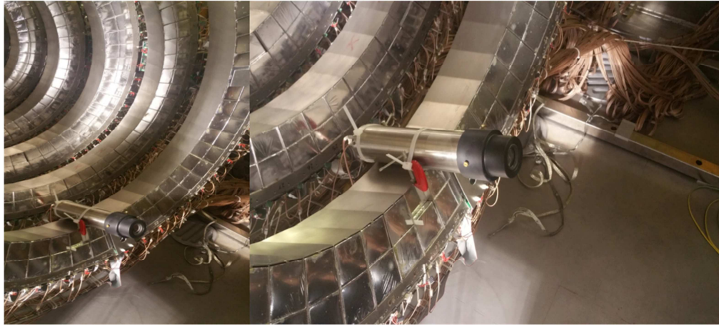
Figure 9: test of the EJ-299-33 close to the sphere of the CHIMERA detector.
