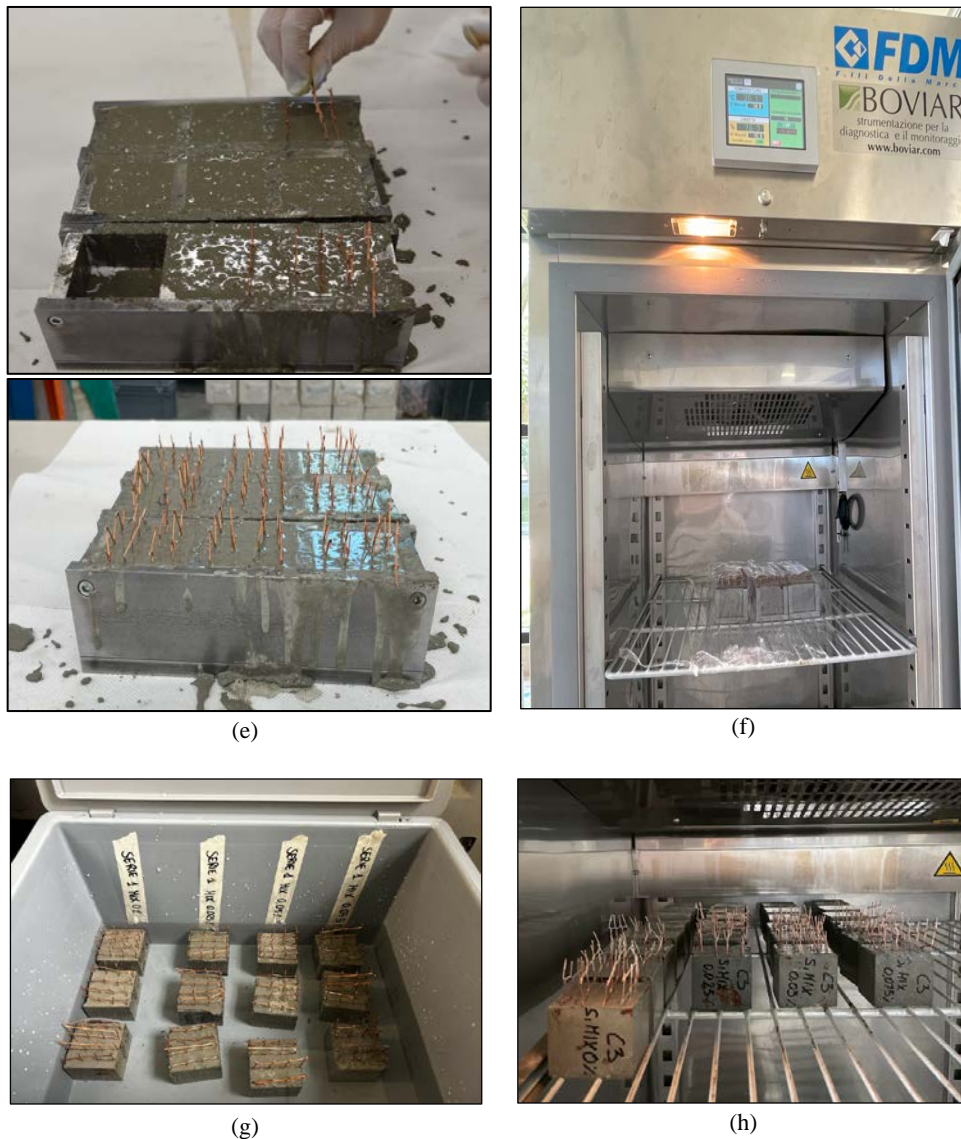
Figure 3.7. Samples preparation steps: (a) addition of the dispersing agent and MWCNTs to water; (b) sonication of the suspensions; (c) mixing of the suspensions with cement powder; (d) vibration of the samples; (e) introduction of the copper meshes into the fresh mixture; (f) storage of the samples; (g) immersion in water; (h) drying phase of the samples.
