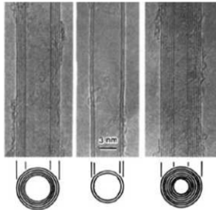
Figure 2.12. Transmission electron microscopy images of MWCNTs with 5, 2 and 7 walls [116].
