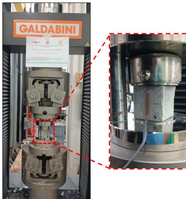
Figure 3.9. Experimental set-up of the compressive strength tests in the second experimental investigation.
