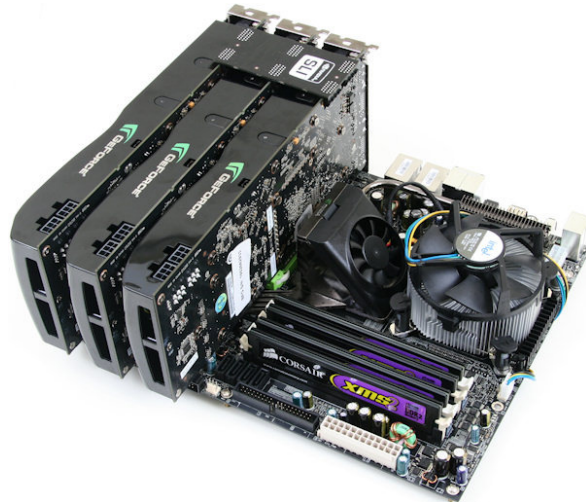
Figure 2.4: A consumer-level multi-GPU workstation reaching the theoretical speed of one TFLOPS
