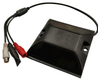
Figure 2. Sensor modified to be buried.
