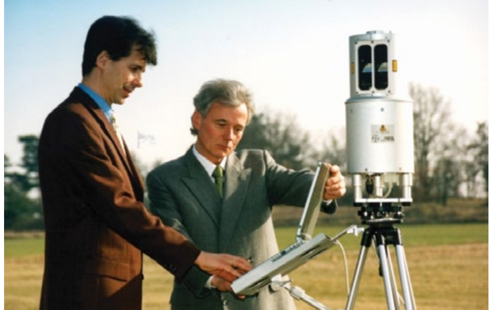
Fig. 3 | Every first-generation scanner that was marketed from 1998 to 2000 was controlled via connection to a laptop. Riegl's original LMS-Z210 is shown with Dr. Andreas Ullrich (left) and Dr. Johannes Riegl (right). Source: https://www.xyht.com/lidarimaging/early-3d-scanning-competition-1998-2000-part-13/
