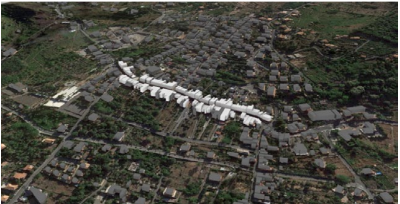
Fig. 4 | Bird's eye view of the model at LOD1. In white the buildings with a known number of floors, in gray the buildings with assumed height.
