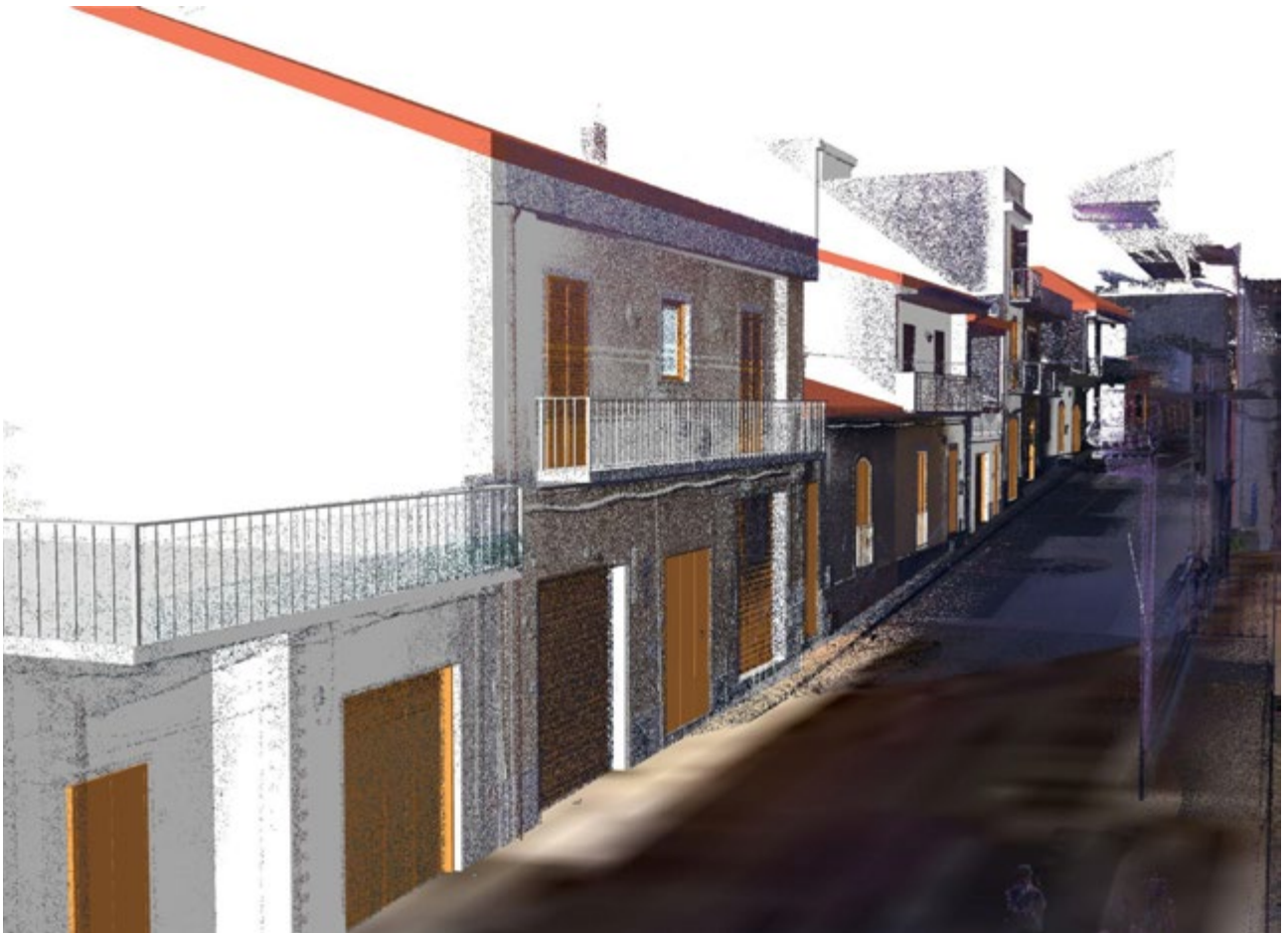
Fig. 14 | Perspective view of the georeferenced point cloud aligned to the CIM model (LOD 3).
