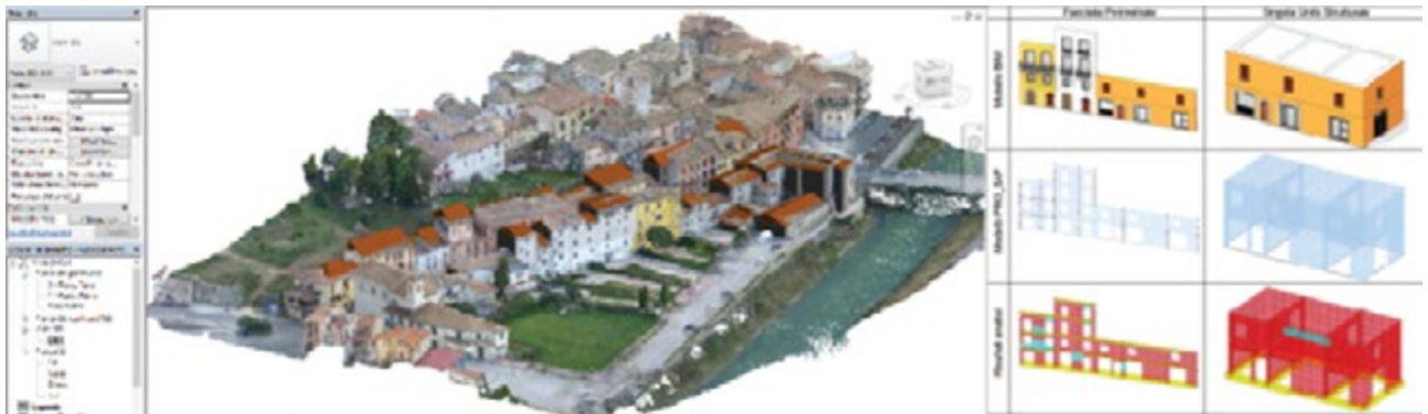
Fig. 45 | Example of BIM-based 3D city model for risk assesment. The methodology applied was called Historical Town - BIM . (Source: Pelliccio et al., 2017)
