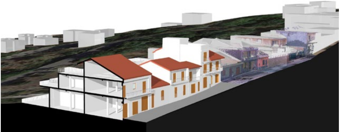
Fig. 16 | View of the final model with supposed internal elements and aligned point cloud.
