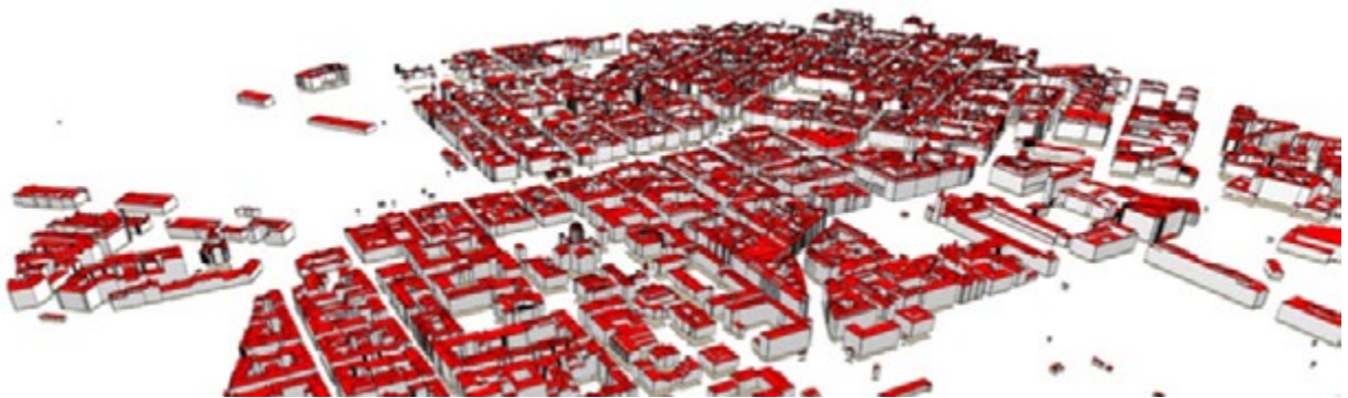
Fig. 46 | CityJSON Building Generation from Airborne LiDAR 3D Point Clouds . (Source: Nys et al., 2020)
