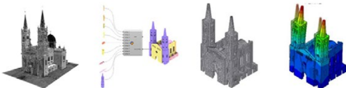
Fig. 31 | Generation of a mesh model for FEM analysis from a NURBS mathematical model generated using point cloud cross sections. Source: Fortunato et al., 2017.
