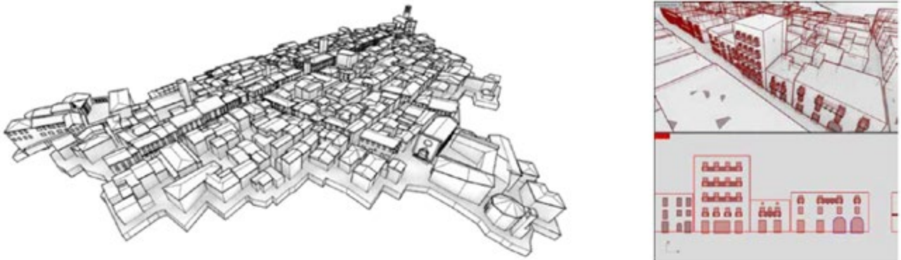
Fig. 47 | 3D reconstruction of the city of Amatrice using Grasshopper and opendata. (Source: Calvano et al., 2019)
