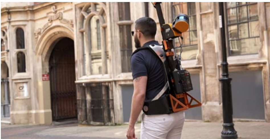
Fig. 6 | ZEB Horizon LiDAR SLAM-based scanner with backpack mobility option for indoor and outdoor mobile mapping. Source: https://www.anivaa.com/buyers-guide/3d-scanners/slam-3d-scanners-imms-mobile-mapping/
