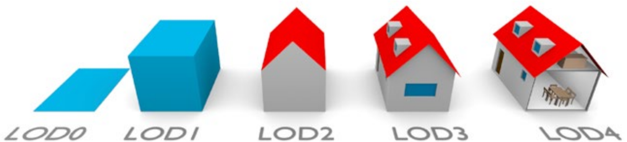
Fig. 35 | The five LoDs in CityGML for the exterior of a building. (Source: Biljecki et al., 2014).
