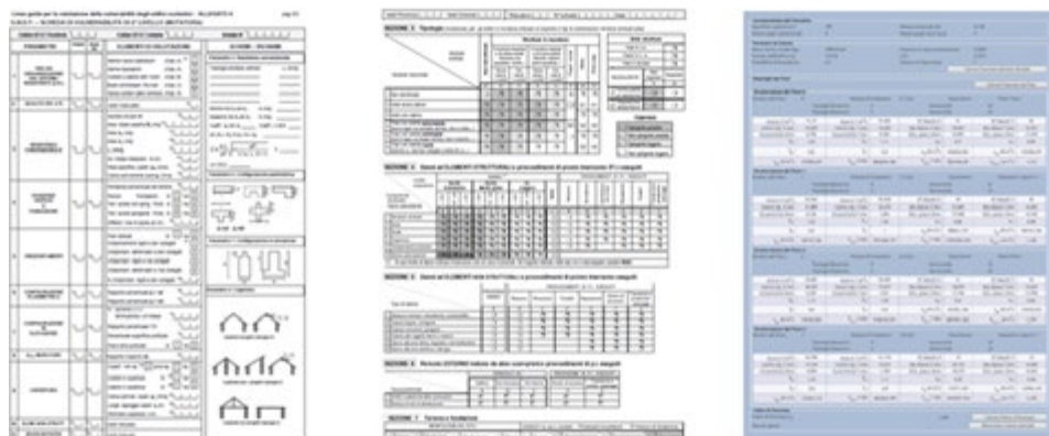
Fig. 1 | Templates used for preventing and managing activities related to seismic risk scenarios (from left to right: GNDT, AeDES, SIVARS). These forms are filled out manually by an operator following predefined procedures. Thus, the validity of these forms depends on the competence of the operator.
