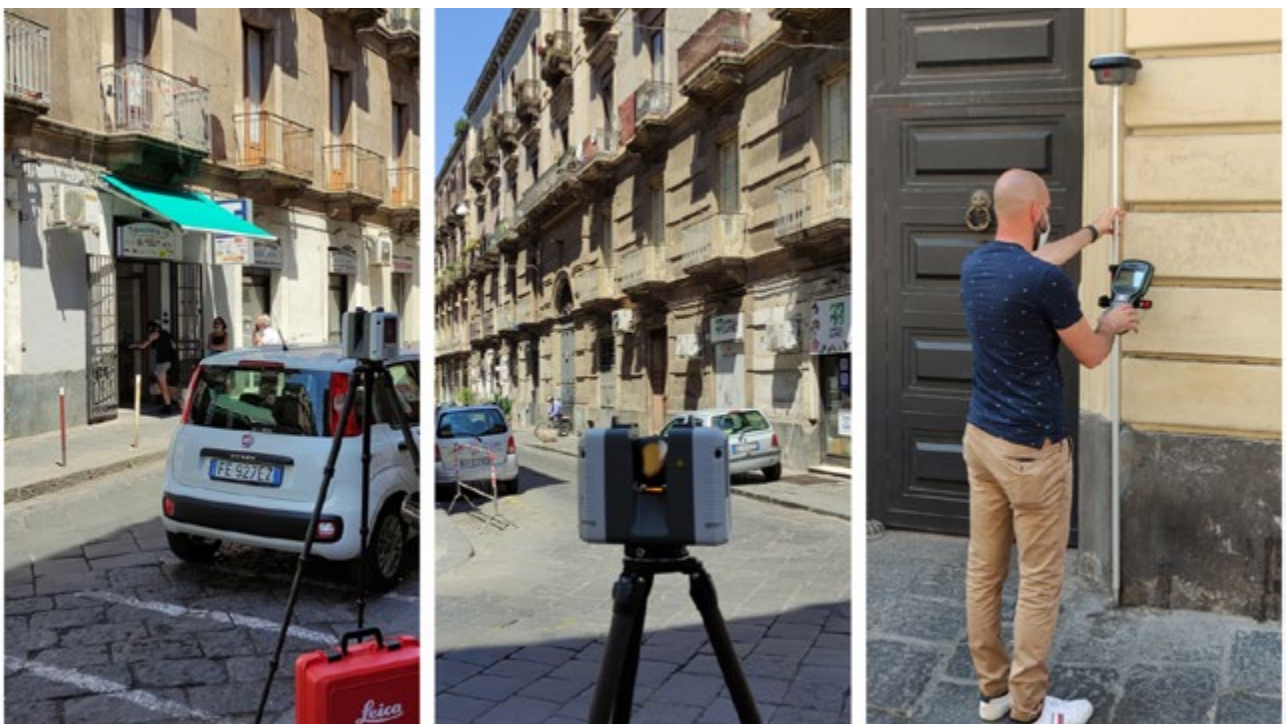
Fig. 40 | Images of the acquisition phase in situ with the Leica RTC360 and GNSS antenna for marking Ground Control Point..
