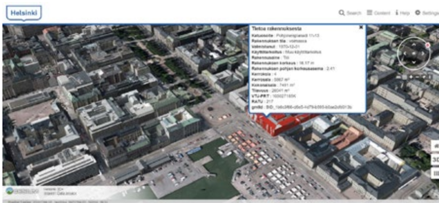
Fig. 43 | View of the three-dimensional information system Helsinki 3D+. It is possible to consult the system both as a CIM (created from geodata, BIM models and laser scanner point clouds) and as a 'Reality Mesh model' (polygonal photogrammetric model obtained from aerial photographs of the entire city). Source: Helsinki 3D+ Information Model. Link: https://kartta.hel.fi/3d/
