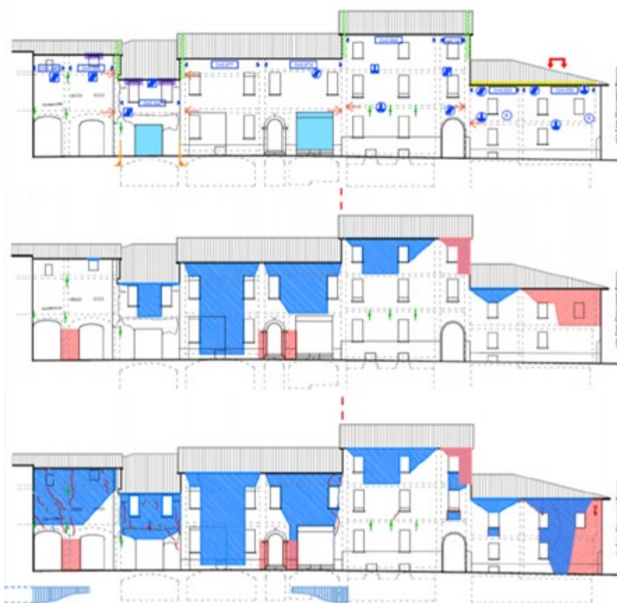
Fig. 27 | Analysis of a sample block in the historic center of Faenza. From top to bottom: critical survey of structural components, vulnerability and strength analysis, damage scenario analysis. Source: Carocci C.F., (2013), Conservation of wall fabric and mitigation of seismic vulnerability. Introduction to the study of aggregate buildings . In: Blasi C. (ed.), Historic architecture and earthquakes. Operational protocols for knowledge and protection . Wolters Kluwer Italy, pp. 138-153
