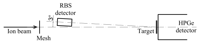
Fig. 4. The scheme of the experimental setup used for the experiment performed in normal kinematics.
