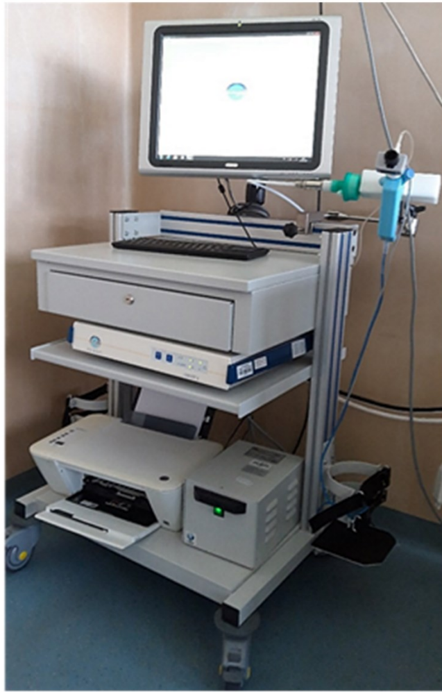
FIGURE 3. MULTIPLE-BREATH N 2 WASH-OUT DEVICE IN OUR DEPARTMENT: EXHALYZER-D (ECO MEDICS AG, SWITZERLAND)
