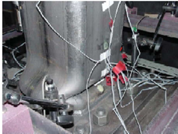
Fig. 20 – Local buckling at the fixed-end section [32].
