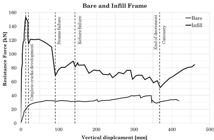
Figure 4.28 Full-height Infill Frame structural response
