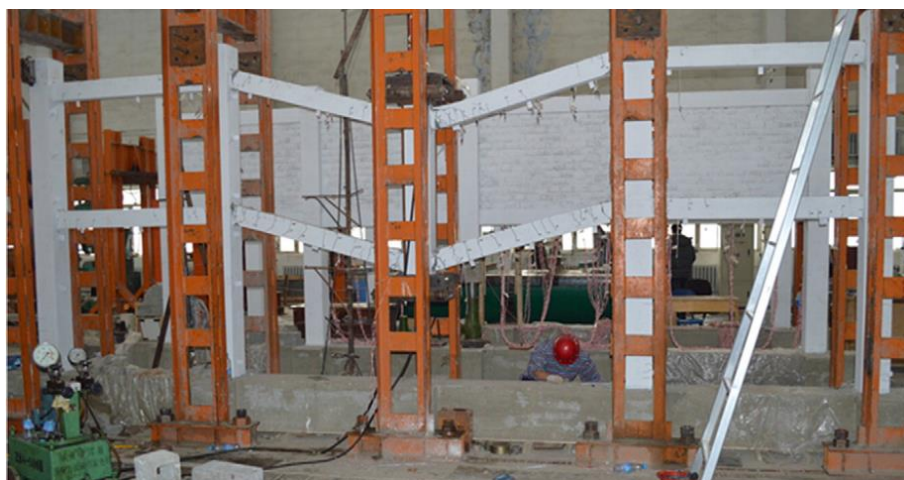
Figure 4.24 (Colour) Collapse shape of the bare frame specimen [49]
