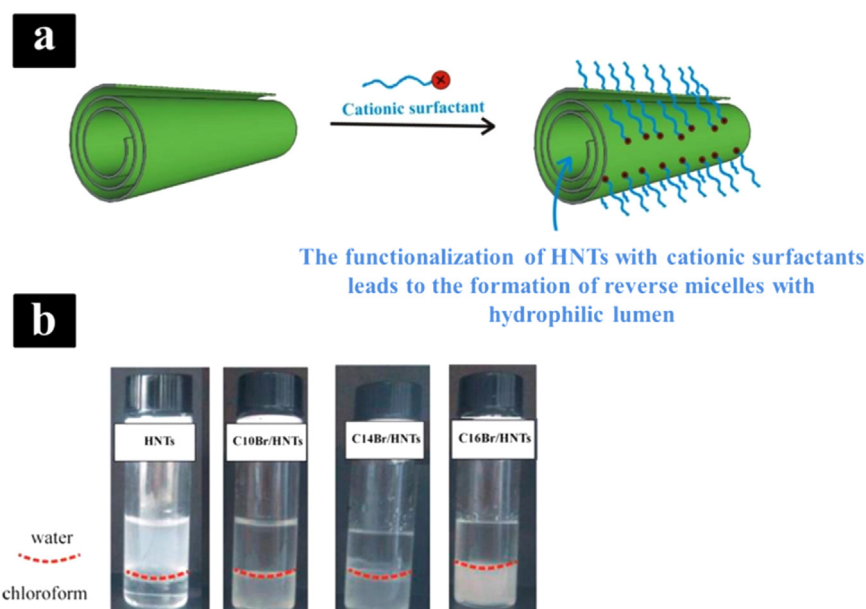
Fig. 5. Scheme of HNTs functionalization with cationic surfactants (a) and partition of pristine and functionalized HNTs between the oil and the aqueous phases (b) adapted with permission from [66], copyright 2015 American Chemical Society.
