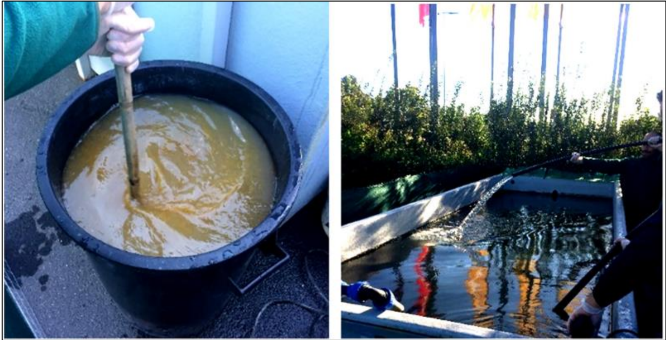
Figure 6.2 - Pilot hybrid-TW system (Catania, Italy): the addition of metals to produce semi-synthetic stormwater runoff (SSR) for the experimental set-up.
