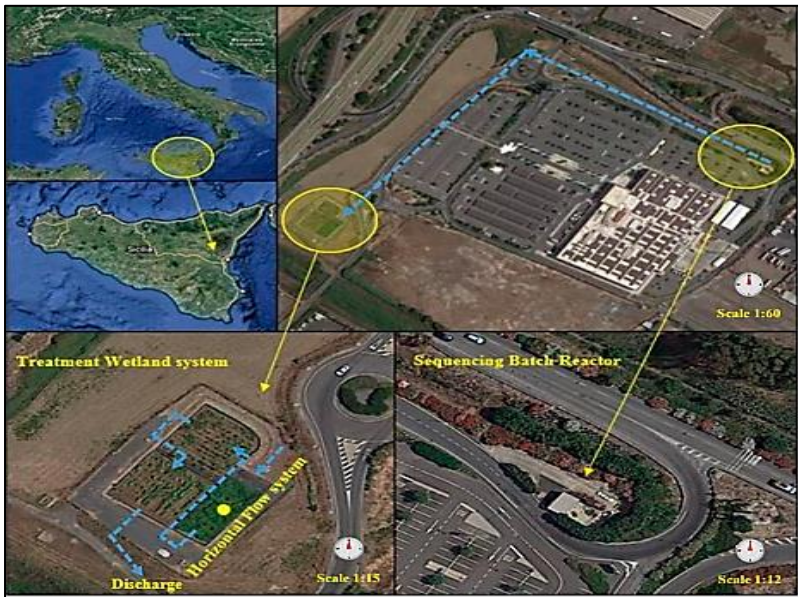
Figure 5.1 - Map of the location area and the hybrid treatment wetland (TW) at the IKEA® store, located in Catania, Sicily, Italy, showing the water flow routes (in blue).
