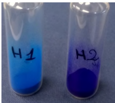
FIGURE 3.6: Hydrated powder samples before the tableting for H1-40 MPa and H2-40 MPa tablets respectively.
