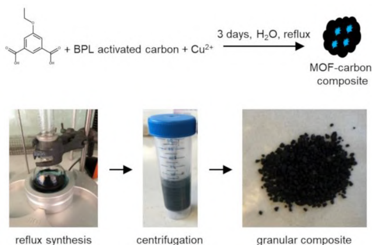
FIGURE 3.10: Main steps of the synthesis of the STAM-17-OEt@BPL composite materials.
