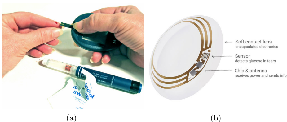
Figure 2.2: (a) A typical kit for glucose self-monitoring, consisting in an enzymatic glucometer and a lancing device, and (b) Google Contact Lens, formed by a miniaturized sensor and a wireless communication system [2.4].
