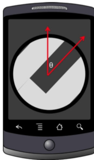
Figure 3.9: Angular shift that lets to calculate the orientation
