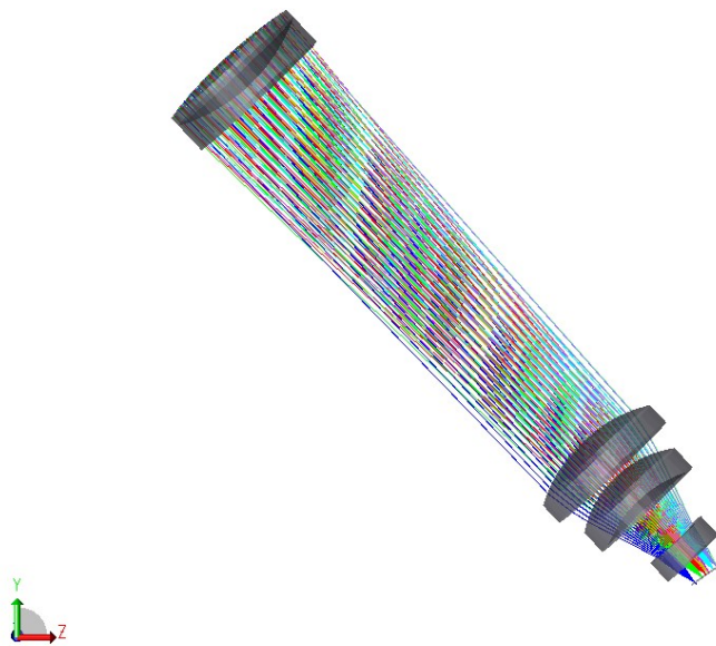
Fig. 3.12.: Optical design of CAOS F/2.1 camera. Note the tilted focal plane to correct for axial chromatism.
