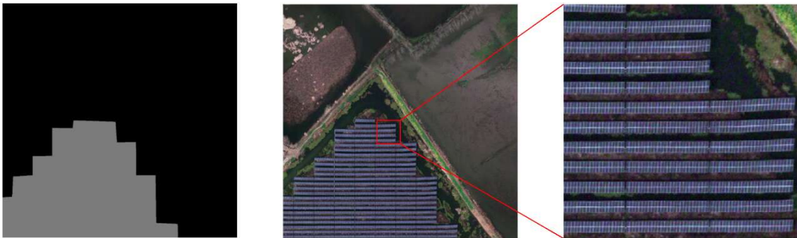
Figure 3.5: The region enclosed by the dataset annotations includes both PV panels and background areas.
