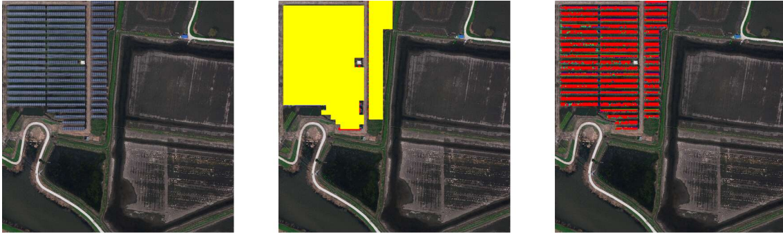
Figure 3.2: Example final outputs of the proposed approach. The original PV image is shown on the left, the detected area for PV panel deployment is shown in yellow in the middle, and the individually detected PV panels are shown in red on the right.
