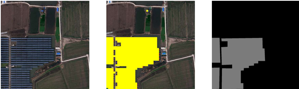
Figure 3.15: Results of PV panel region detection (middle) compared with the original dataset label (right). The original image is shown on the left for reference.
