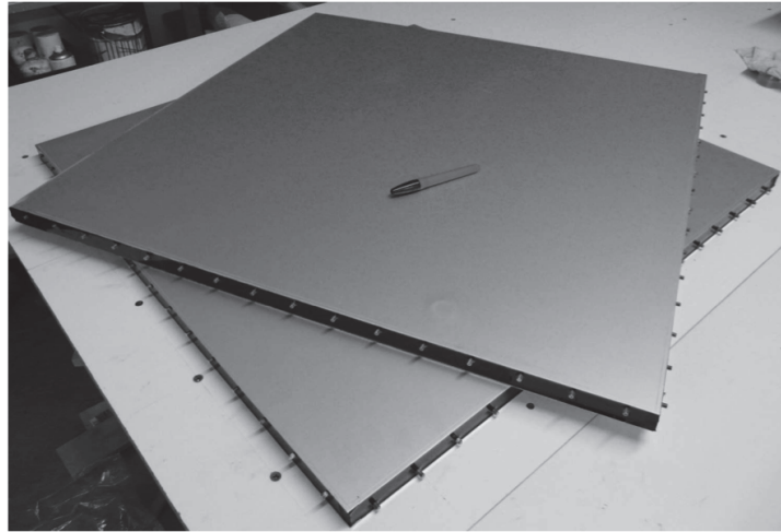
Figure 1.11: View of the two 16 \times 16 matrices [24]. The optical plugs are visible on two sides of each matrix and are to be connected to the clear fibers guiding the light onto the channels of the photomultiplier. The thickness of the matrices is 27 mm and their individual total weight is 20 kg.
