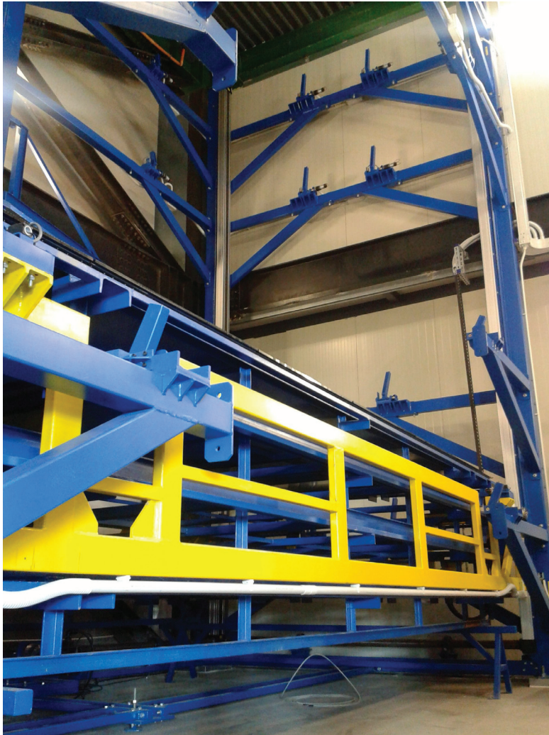
Figure 2.5: Picture of the actual mechanical structure of the Muon Portal detector. The structure, which can be controlled through an electrical panel, consists of movable planes (blue) which, once placed via the elevator (yellow) to the loading position, will be hooked up through the use of pistons automatically handled.
