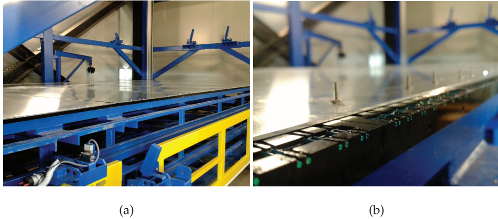
Figure 2.6: Picture of the first logical plane (X-Y) which has been recently assembled and positioned on the mechanical structure (a), particular (b).
