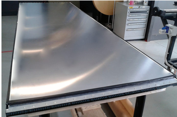
Figure 2.25: Picture of the completed module. The side with cookies and fibers is visible.
