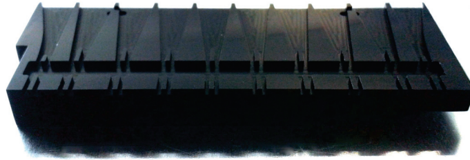
Figure 2.22: A black PVC adapter (cookie) specifically designed for the project in order to ensure the desired fibers positioning so that they can be optimally coupled with the SiPMs.
