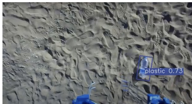
FIGURE 17. UGV waste localization and recognition on the field (Ramla Bay in Gozo, Malta).
