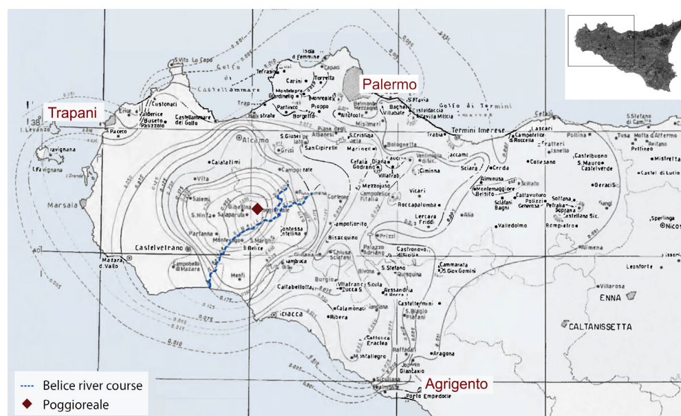
Figure 2. Map of “Isoblaste” (equal damage contour levels) for the 1968 earthquake. Highlighted are the Belice River that crosses the territory and the provinces of Palermo, Trapani, and Agrigento affected by the seismic event.
