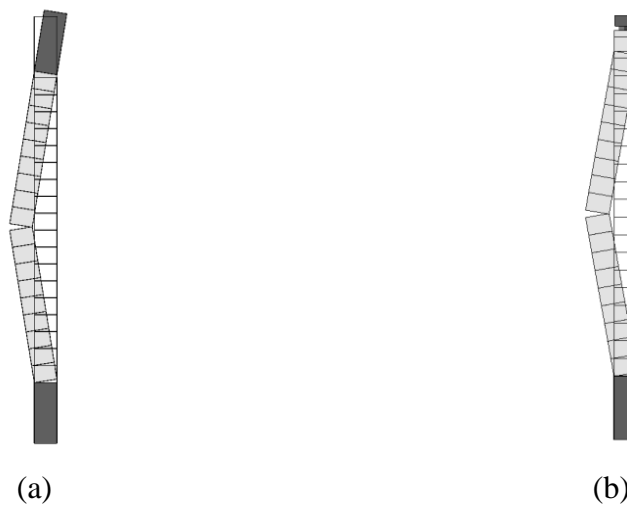
Figure 51 - Collapse mechanisms for : (a) \sigma_v = 0 MPa; (b) \sigma_v = 0.15 MPa
