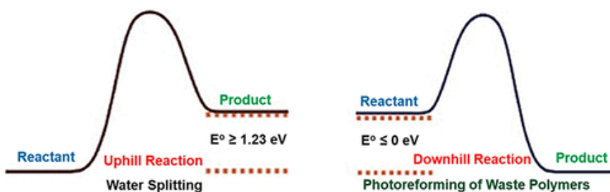
Figure 5 Water splitting is an endothermic process, while photoreforming of waste polymers is exothermic [36].
