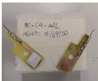
FIGURE A.9: BC-Ch-Mal degraded membrane
