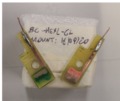
FIGURE A.6: BC-HEXYL-CL degraded membrane
