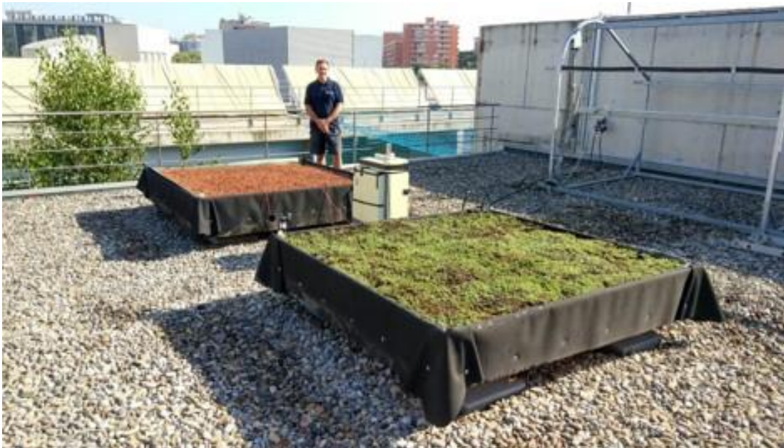
Experimental set-up for passive cooling assessment at the University of Lleida, Spain
