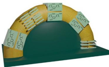
Figure 3.10. Schematic picture of the conformal adhesion of the polymeric lamellae on the nano-curved surface, leading to the progressively changing orientation of both face-on and edge-on lamellae with respect to the substrate baseline (The figure is not scaled, and it does not represent the actual arrangement of lamellae on nano-curved substrates).
