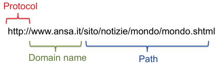
Figure 2.1: Components of a URL: protocol, domain name and path of a Web resource.
