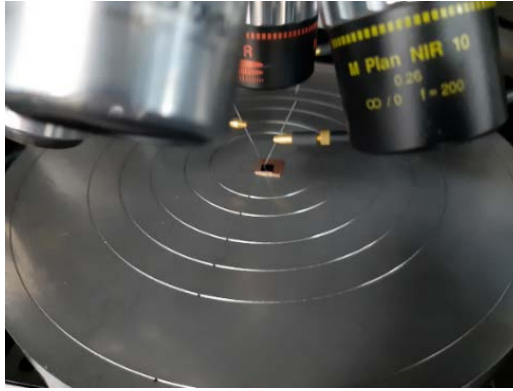
Figure 3.3.1: Two- point probe measurement performed on the 4H-SiC p-n junction.
