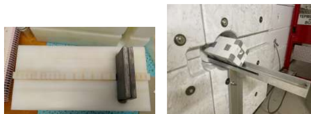
Figure 7: Distribution of the gold foils inside ANTILoPE together with the Pb block (right) and the complete set-up placed just after the NEAR collimator (left).
