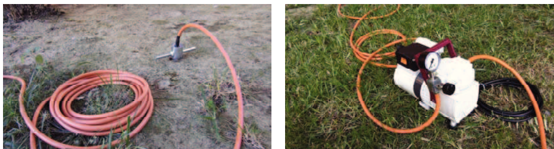
Figure 4.5 - Drilling rod hit at 1 meter depth into the ground (left picture) and pump to convey the soil gas into the laboratory facility (right picture).
