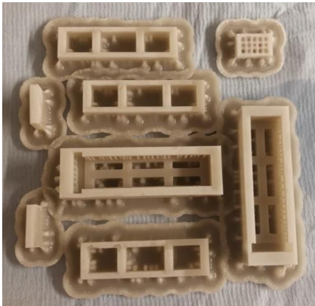
Figure S1 The 3D printed cage component precursors. After trimming and polishing, the cage components were baked to remove the wax composition in the resin and partially anneal the SiO 2 to get an integrated part (1100°C resistance).
