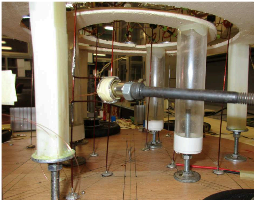
Figure 16 - Actuators in correspondence of an abutment of the inner circumference.
