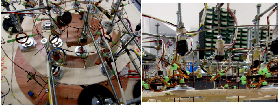
Figure 11 - TCRT5000 reflective optical sensors monitor the phase of each rotating coil
