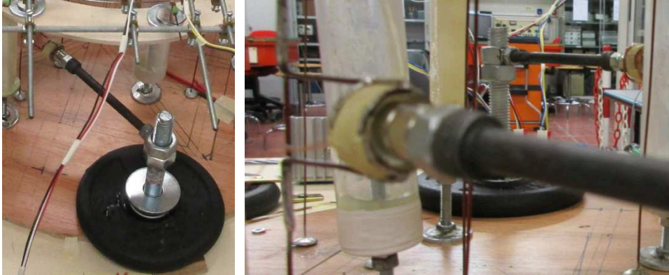
Figure 12 - Couple of electromagnetic actuators are used to activate the circular structure.
