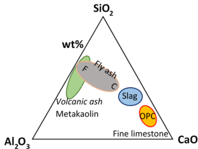
Fig. 1.8 - \text{CaO-Al}_2\text{O}_3\text{-SiO}_2 ternary diagram of cementitious materials. Abbreviation: OPC- Ordinary Portland Cement.
