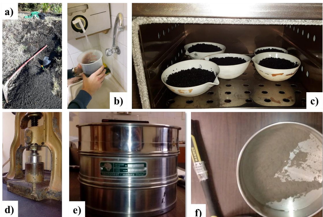
Fig. 2.2– Sampling and treatments of raw materials: a) sampling of volcanic ash in Santa Venerina landfill; b) cleaning step with distilled water; c) drying step into oven; d) press machine
