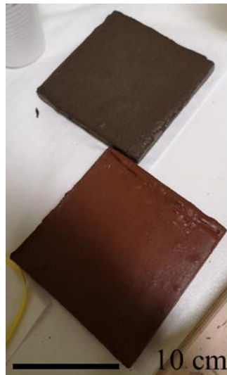
Fig. 7.1 – Tiles just removed from the mould.
