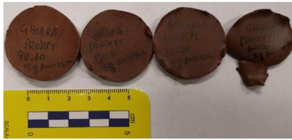
Fig. 7.2 - Samples prepared to estimate the curing time at increasing prompt amount.
