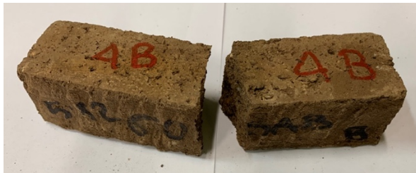
Figure 6 - Failure mode of specimens
