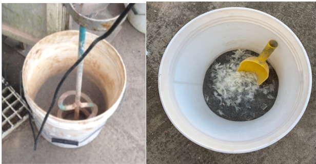
Figure 3 – mix preparation, and addition of SWF into the mix
