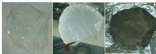
Figure 4. 9 From left to the right: Nafion, Nafion- \text{TiO}_2 and Nafion with GO-based materials.
