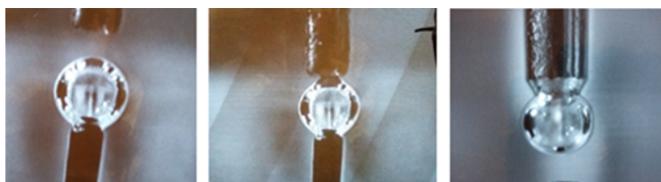
Figure C.1: Bubble formation and anchoring to an upper electrode.
