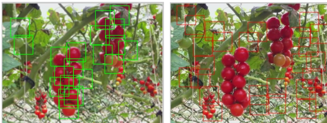
Figure 154 - 20 True Positives against 26 False Positive with threshold of 0.2
