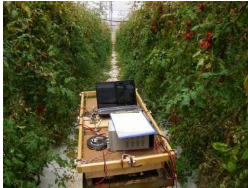
Figure 118 - The experimental setup with eight SFR08 sensor modules
