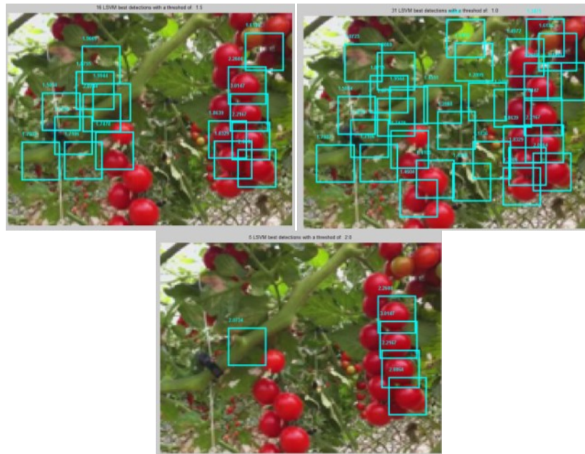
Figure 144 - Detection varying the threshold: 1, 1.5 and 2 (Test_Image_1)
