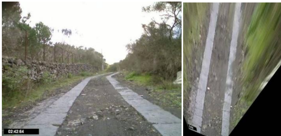
Figure 42 - Original image (on the right); reconstructed top down “bird’s eye” view (on the left)
