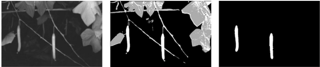
Figure 16 - Detection of cucumber fruit using computer vision. Original image taken by the camera mounted on the vehicle (left), segmented image (middle) and detected fruit (right).
