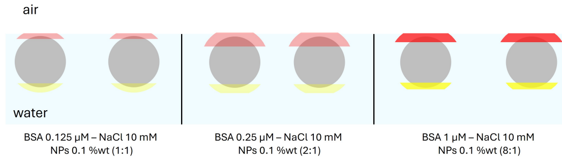
Figure 5.8: In scale illustration of the geometrical distribution of the BSA-NP complexes adsorbed at the air-water interface as obtained by NR fitting with the physical model described in Section H.5. In gray are represented the silica nanoparticles, in red the air-facing BSA shell, and in yellow the water-facing one. The different BSA shell composition in terms of protein dry fraction \phi_{BSA,i} are reported as differences in the color transparency. The illustration helps to visualize the empty space between BSA-NP complexes.
