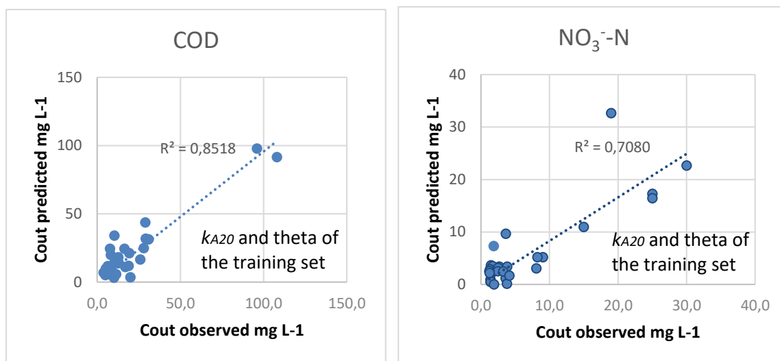
Figure 4.4: COD (mg L -1 ) and NO 3 - -N (mg L -1 ) – Predicted Vs Observed values
