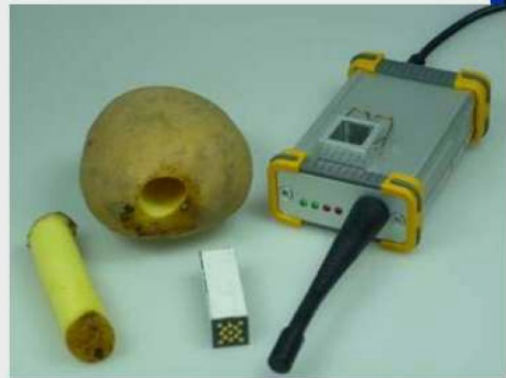
Figure 1.3: Specification and view of miniaturised acceleration measuring unit (AMU) and its implantation in potato tuber (Praeger et al., 2013).
