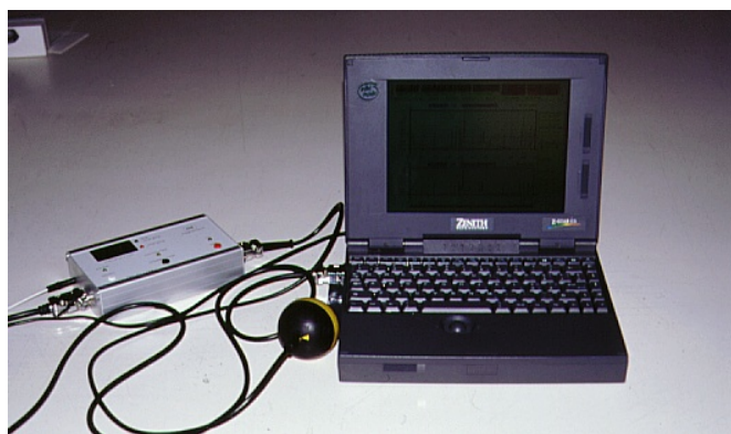
Figure 1.2: Instrumented Sphere PMS 60 developed at ATB.
