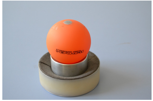
Figure 3.4: Positioning of the sphere for measuring the modulus of Young.
