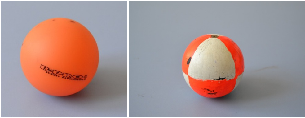
Figure 3.1: The two artificial fruits used for the drop tests: BALL 1 (left) and BALL 2 (right).
