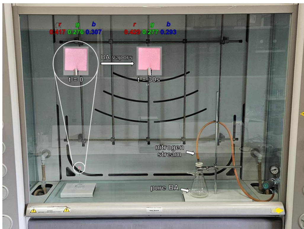
Figure 4.24. Experimental setup for simulating an accidental release of BA vapors within a semi-confined space in the presence of annealed 1-PBF1s. Pure BA (10 mL) is contained in a sealed conical flask (volume = 500 mL). The conical flask is connected to a continuous nitrogen stream operating at 0.5 bar in order to force the evaporation of BA. The glass tail (diameter = 5 mm) of the conical flask acts out the escape of BA vapors. The annealed 1-PBF1 is placed 60 cm from the BA steam outlet and monitored over time.
