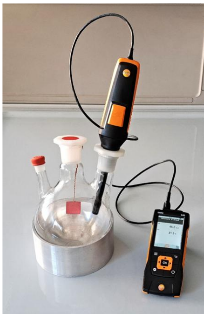
Figure 3.1. Experimental apparatus for static exposure of PBFs to VOC vapors.
