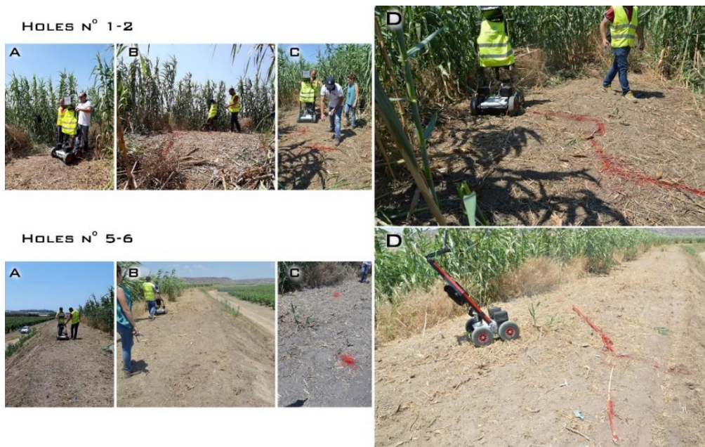
Figure 4-29: GPR survey for holes 1-2 and 5-6: A) GPR position on the levee crest; B) GPR scans; C) Record soil discontinuity; D) Reconstruction of burrow path inside the levee.
