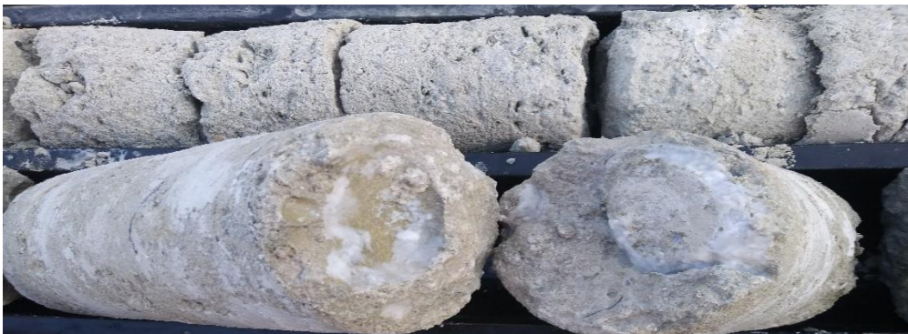
Figure 7-28: core drilling to evaluate the chemical mixture performances.
