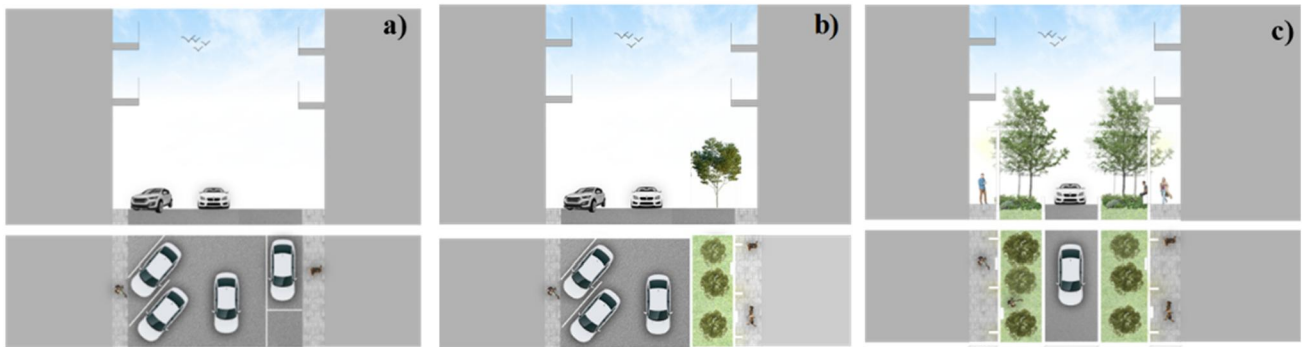
Figure 3.13. Cross sections of the roads: a) Existing configuration; b) and c) Design scenario.
