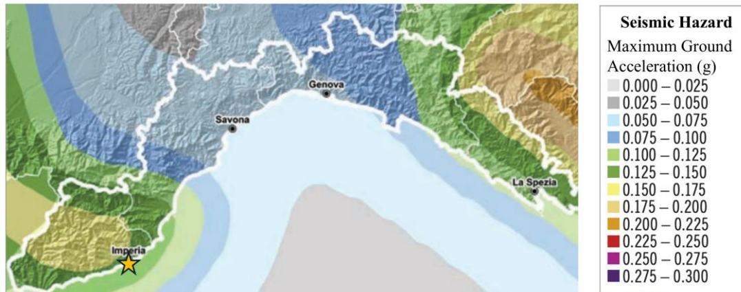
Figure 2: Seismic hazard in Liguria (MPS04, http://zonesismiche.mi.ingv.it/ ). The star indicates the location of the Bussana village.
