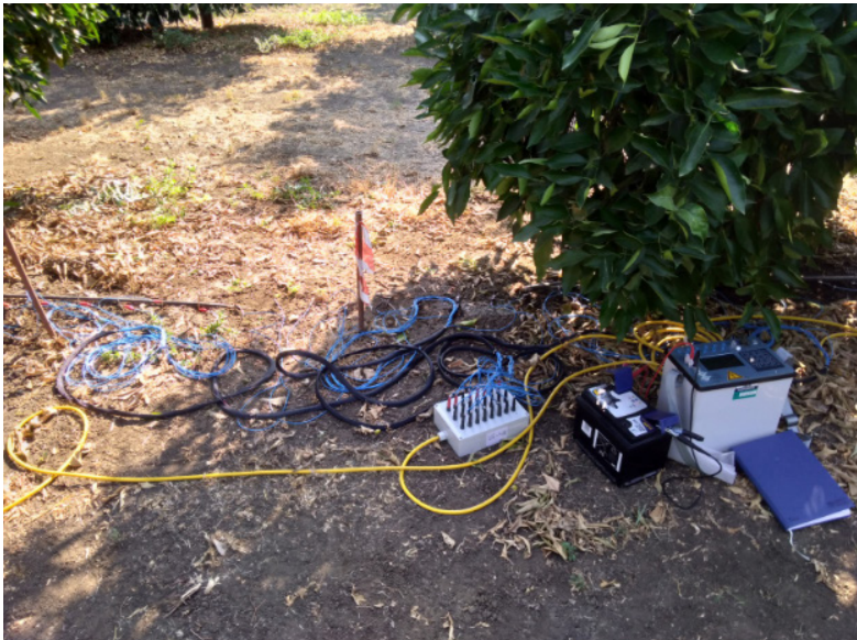
Figure 4. Field equipment electrical resistivity tomography
