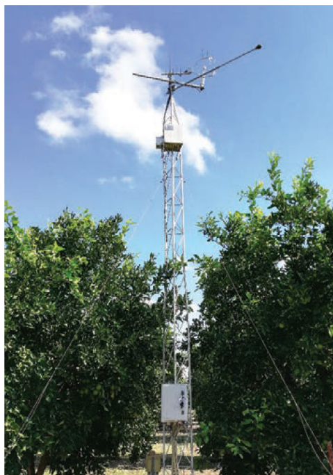
Figure 1. Micrometeorological tower installed at the experimental site.
