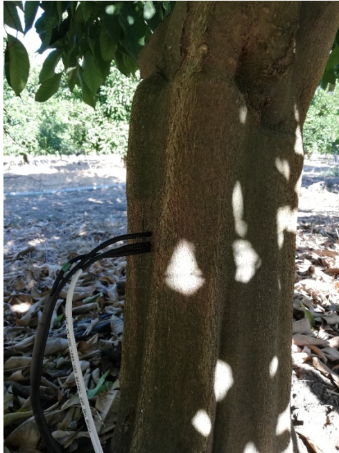
Figure 8. Heat Pulse Velocity technique. Heat pulse thermistore and heater installed in sapwood of tree
