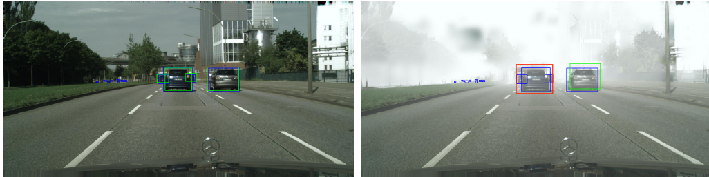
(b) Training on sunny images and testing on sunny (left) and foggy (right) images. The detection results show incorrect bounding box predictions, pointing out the impact of environmental variations on performance.
