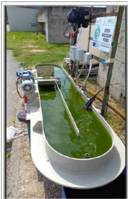
Figure 3 - Pilot station for wastewater based on microalgae
