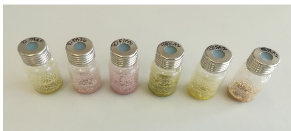
Figure 20. Vials with ground tissues dissolved in EDTA (50 mM) and CaCl 2 (5 M) solution.
