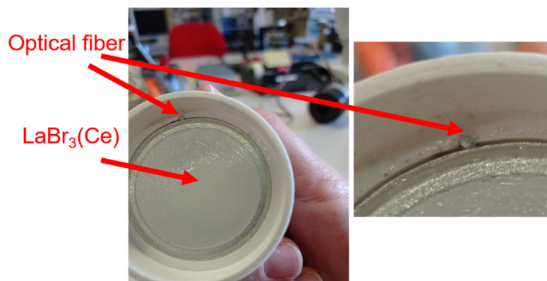
Figure 10. Details of the experimental setup for the laser measurement. The optical fiber is installed sideways with respect to the LaBr 3 (Ce) crystal. The laser light is sent through the optical fiber directly to the window of the PMT.
