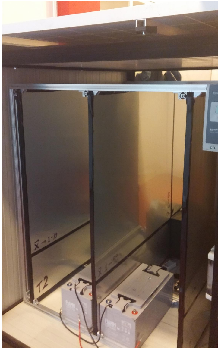
Figure 1.1: Assembly phase of the telescope. It is possible to see the three sensitive planes fixed vertically on an aluminum frame to keep the alignment inside the external box.
